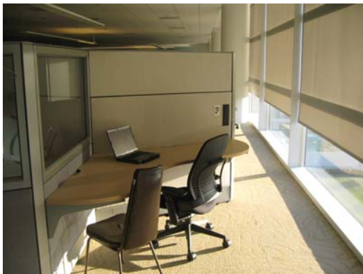
Desks are 3 ft from window requiring shades to be down limiting the ability to daylight
